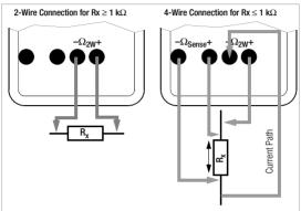
Zero Balancing for the " $\Omega_{2W}$ " and " $\Omega_{4W}$ " Functions
